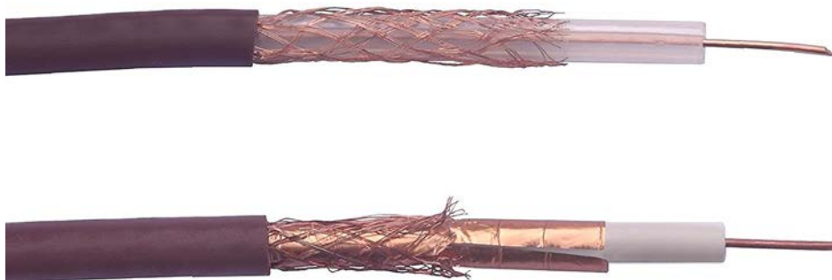
Two types of low-cost coaxial cables were tested: one with a shield comprising only a 40% coverage braid shield (top), and one with a shield comprising a foil plus braid (bottom).
